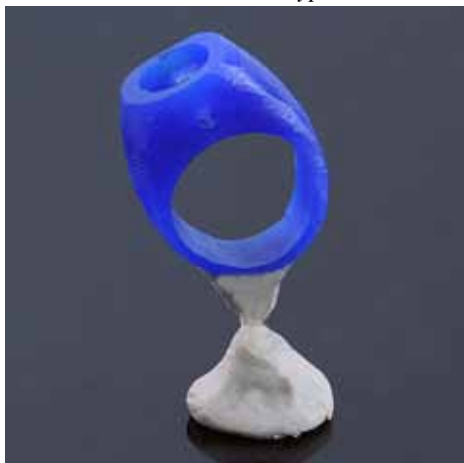
Fig 2. Lost wax modeling often done with heat After the wax model is created, it is "sprued" which means it is placed on a soft wax pedestal and cylindrical can is placed over the object. The can is filled with "casting material" (usually a high temperature plaster), and allowed to harden. The wax is then burned out of the plaster in an oven, leaving behind a perfect mold of the object. The "sprue" becomes the entrance funnel for pouring the metal.
