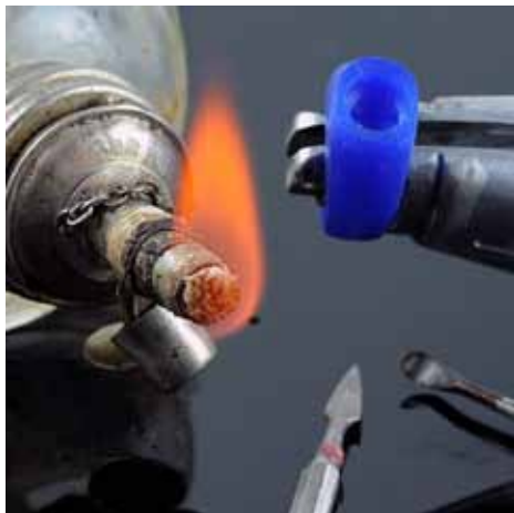
Fig 1. Lost wax modeling often done with heat and dentist type tools.
