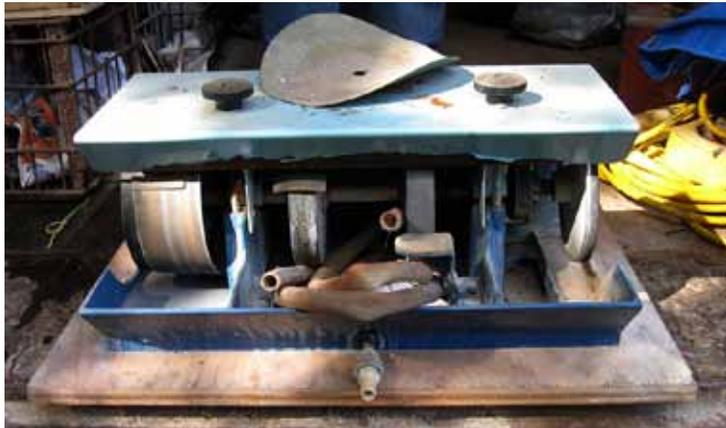
*large -heavy duty - cabochon cutting machine with room for two wheels, two expanding drums and spin-on polishing disk*
