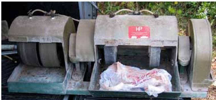
*8" very heavy duty capping unit. room for two grinding wheels, and two side by side expanding drums - with end polisher*
